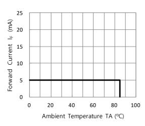
Fig. 2 FORWARD CURRENT VS. DERATING CURVE
